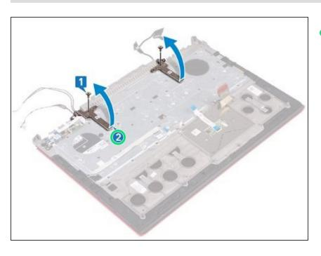
Open the display hinges at an angle of 90 degrees.
