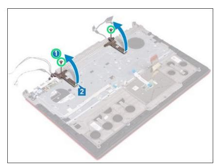
Replace the two screws (M2.5x5) that secure the display hinges to the palm-rest assembly.
