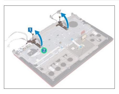
Close the display hinges at an angle of 90 degrees.
