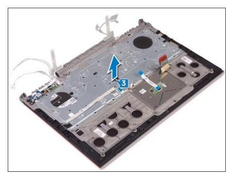
Place the palm-rest assembly on the display assembly.
