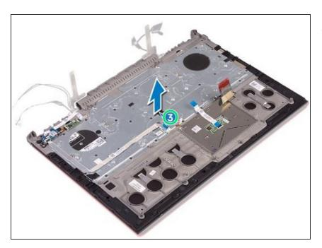
Lift the palm-rest assembly off the display assembly.
