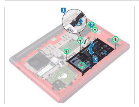
Remove the five screws (M2x4 T8) that secure the battery to the computer base.
