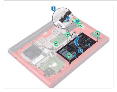
Replace the five screws (M2x4 T8) that secure the battery to the computer base.
