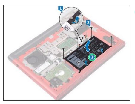
Slide the battery in the slot on the computer base and align the screw holes on the battery with the screw holes on the computer base.
