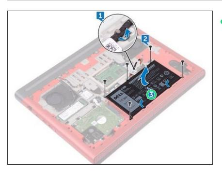
Lift the battery at an angle off the computer base.
