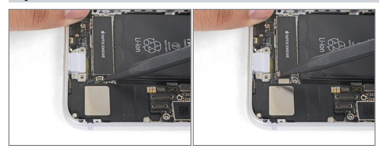
• Use the point of your spudger to pry the antenna cable socket up and away from the connector below it.
