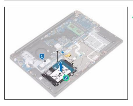
Lift the hard-drive assembly off the palm rest and keyboard assembly.
