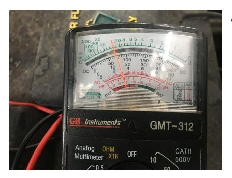
Checked the voltage on the battery terminal with engine running. Shows properly between 14V - 15V
