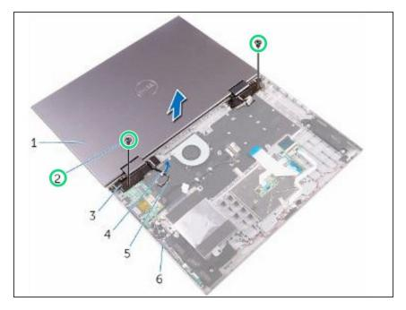
Replace the two screws (M2.5x7) that secure the display assembly to the palm rest and keyboard assembly.
