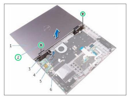
Remove the two screws (M2.5x7) that secure the display assembly to the palm rest and keyboard assembly.
