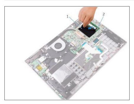
Align the notch on the memory module with the tab on the memorymodule slot.
