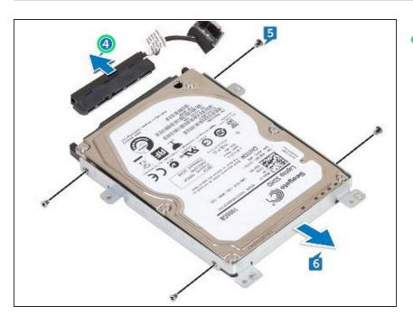
Disconnect the interposer from the hard-drive assembly.
