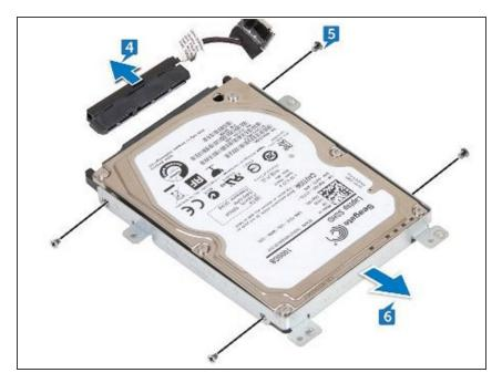
Align the screw holes on the NEW hard-drive bracket with the screw holes on the hard drive.
