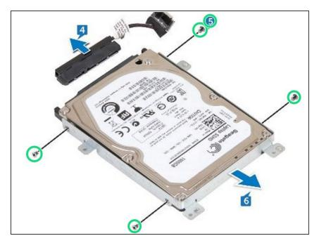
Remove the four screws (M3x3) that secure the hard-drive bracket to the hard drive.
