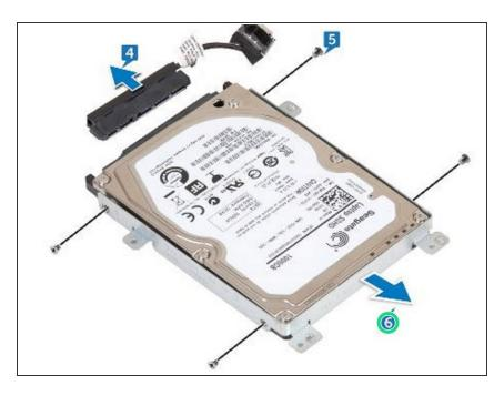
Remove the hard-drive bracket off the hard drive.
