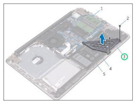
Lift and remove the battery bracket.
