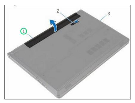
Using your fingertips, lift the battery at an angle and remove the battery off the computer base.
