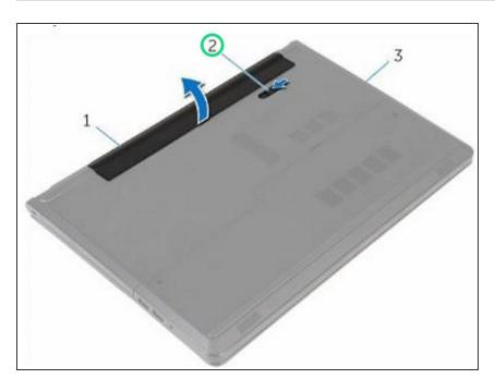
Slide the battery latch to the unlocked position.
