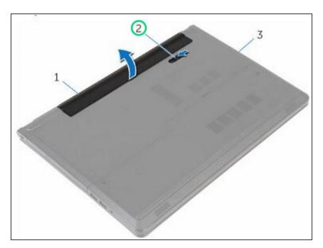
Slide the tabs on the battery into the slots on the battery bay and snap the battery into place.
