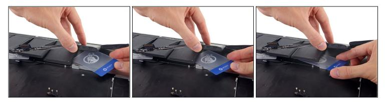
• Repeat the above procedure to separate the last remaining battery cell from the MacBook Pro's upper case.
