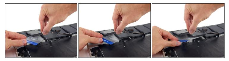
• While lifting the plastic frame out of the way, push one corner of your plastic card underneath the outside edge of the first center battery cell.
