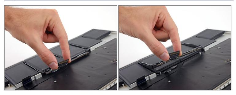
• Grab the battery connector or the top edge of the plastic battery frame and lift it slightly, exposing the top edge of the two center battery cells.
