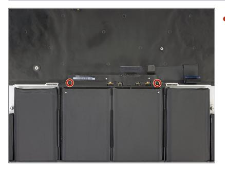
• Remove the two 3.9 mm T5 Torx screws securing the battery board.
