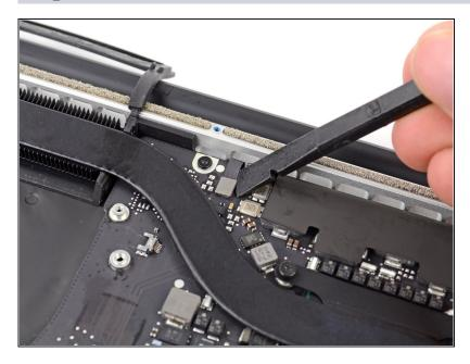
• Use the flat end of a spudger to pry the keyboard backlight connector up from its socket on the logic board.
