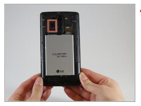
Using a plastic opening tool or your fingers, eject the SIM card from the device.
