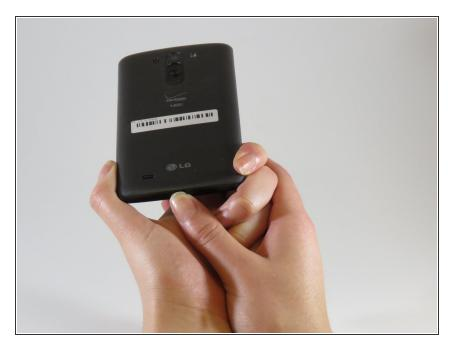
Using your fingers or a plastic opening tool, remove the back cover from your device.
