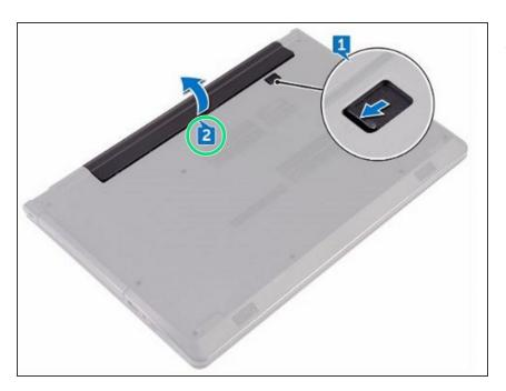
Place the battery in the battery bay and snap the battery into place.
