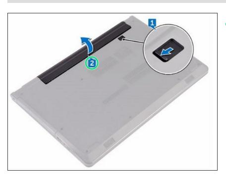
Using your fingertips, lift the battery at an angle and remove it from the battery bay.
