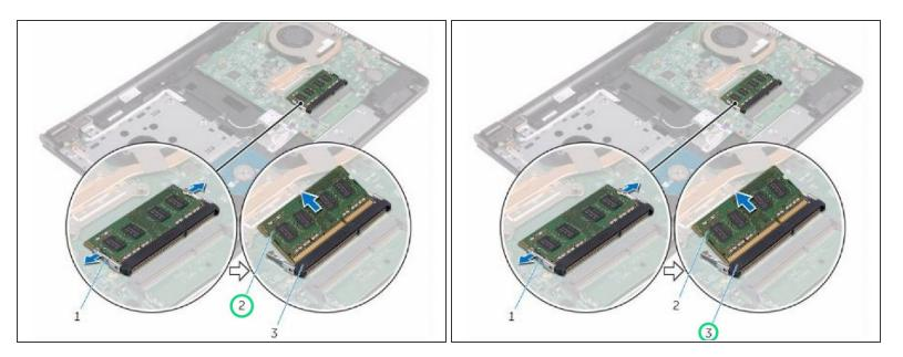
Slide and remove the memory module from the memory-module slot.
