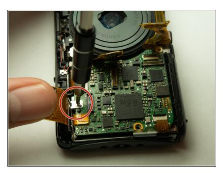
Remove the 3mm Phillips #000 screw from the motherboard.
