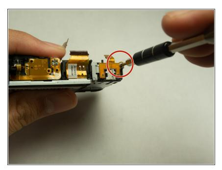
Remove the 3mm Phillips #000 screw located at the top right of the USB port.
