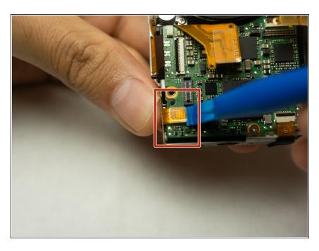
Pry the golden ribbon cable attached to the USB port using a plastic opening tool.
