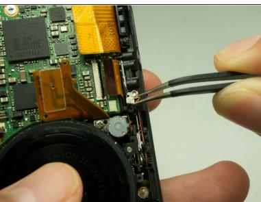
Unplug the small chip from the face of the camera using a pair of tweezers.
