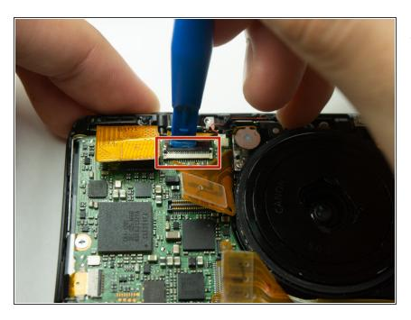
Use a plastic opening tool to flip up the retaining flap on the ribbon cable ZIF socket.
