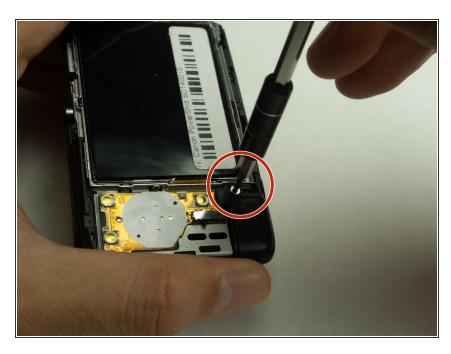
Remove the 3mm Phillips #000 screw from the rear face of the camera.
