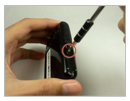
Remove the single 4mm Phillips #00 screw from the bottom.
