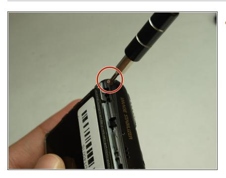
Remove the 3mm Phillips #000 screw from the top of the camera.
