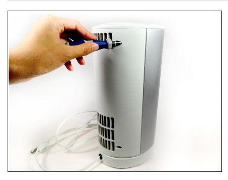
Use the Phillips #2 screwdriver to remove the four 6 mm screws by unscrewing counterclockwise.
