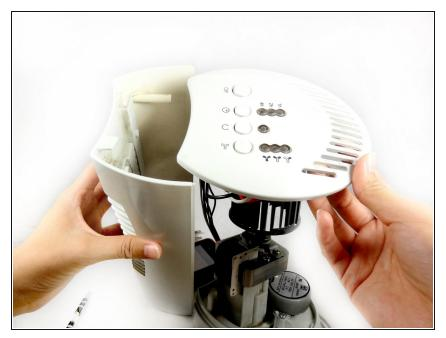
Remove the top cover containing the circuit board and the wires by pulling it away from the outer shell of the fan.
