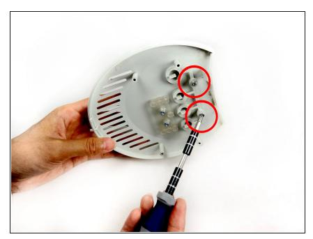
Remove the two 8 mm screws that attach the buttons to the top cover of the fan.
