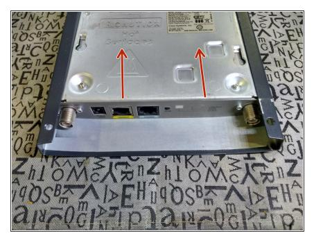
Once the 4 screws are removed, push to the side to remove the cover.
