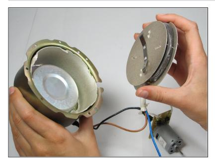
• Remove the heating coil out of the heating component.
