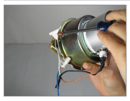
• Unscrew the three 10 mm Philips #2 screws that hold the heating component together.
