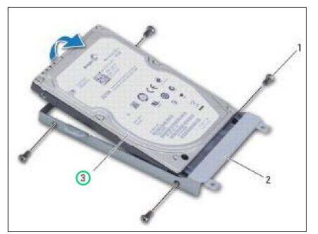
Place the NEW hard drive in the hard drive bracket and replace the four screws that secure the hard drive bracket to the hard drive.
