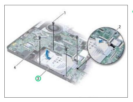
Slide the hard drive assembly into the computer base until it is fully seated.
