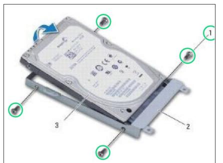
Remove the four screws that secure the hard drive to the hard drive bracket.
