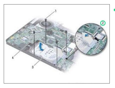
Connect the USB/audio cable to the USB/audio board.
