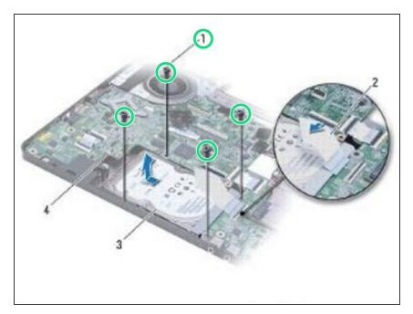
Remove the four screws that secure the hard drive assembly to the computer base.
