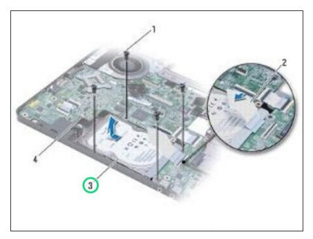
Replace the four screws that secure the hard drive assembly to the computer base.
