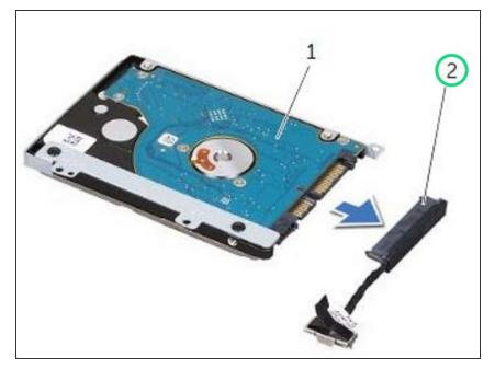
Pull the interposer to disconnect the hard-drive cable from the hard-drive.
