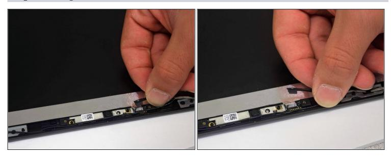
Unplug the connector. It is located on the top of the screen attached to the camera assembly.
