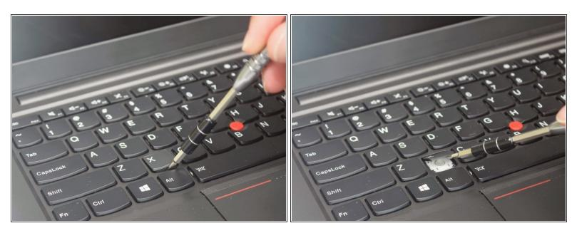
Slide under the key using a flat object and pop it out of place.
