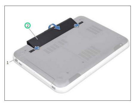
Align the tabs on the battery with the slots on the battery bay and snap the battery until it clicks into place.
