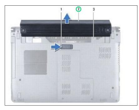
Slide the NEW battery into the battery bay, then push to click the battery into place.
