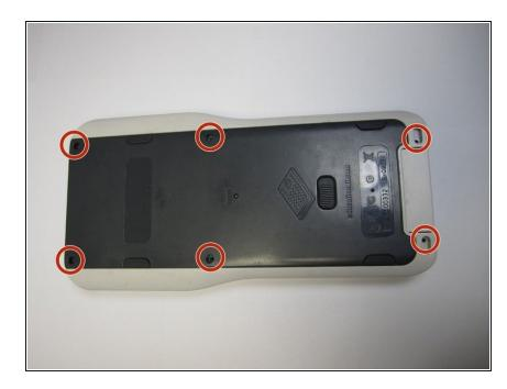
Remove the six 7.3 mm screws from the back of the calculator using a Phillips #000 screwdriver.
