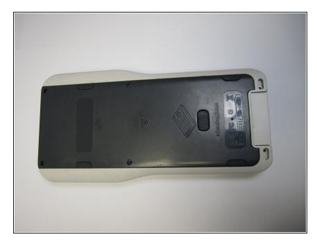
Place the calculator screen facing down, with the back plate facing up.
