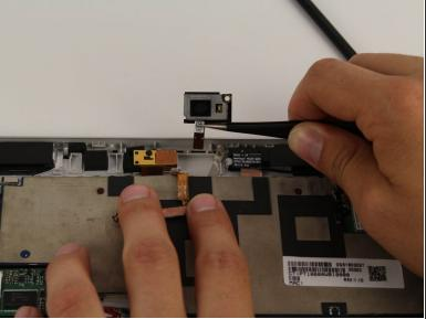
Use a pair of tweezers to disconnect the flex cable from the motherboard and remove the rear facing camera from the device.
