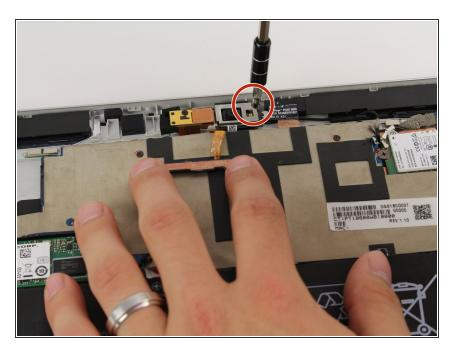
Use a Phillips #00 screwdriver to remove the screw in the corner of the camera.
