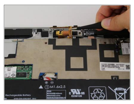
Use a pair of tweezers to remove the flex cable on the top of the camera.
