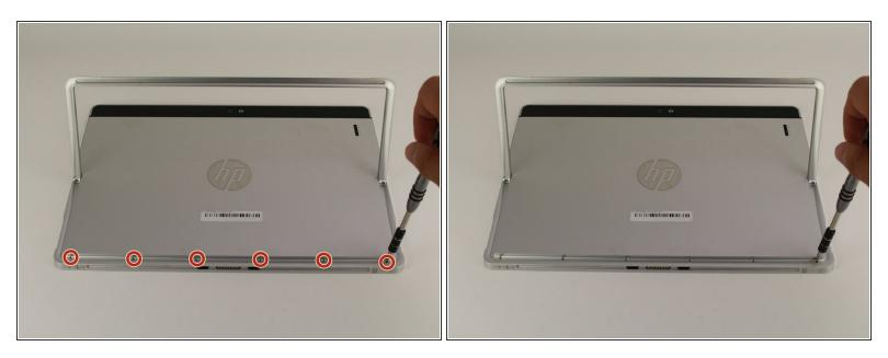
Use a T5 driver to remove the six screws on the back of the tablet.
