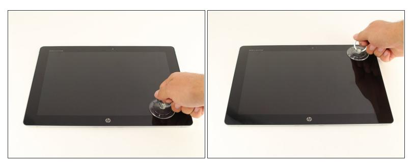
Use the suction cup to carefully separate the screen from the device. Pull upwards with a fluid and smooth motion.
