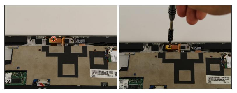
Use a Phillips #00 screwdriver to remove the screw.
