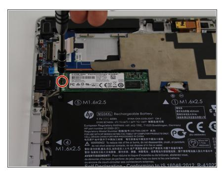
Use a Phillips #0 screwdriver to remove the screw on the left hand side of the card.
