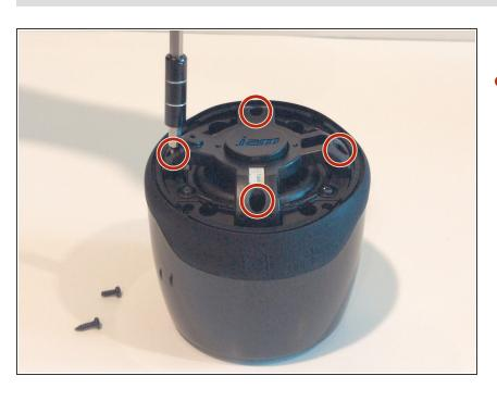
Remove the four 7mm Phillips screws from the plastic cover.
