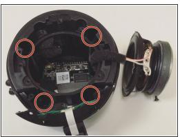
Remove the four 7mm Phillips screws to expose the motherboard.
