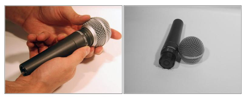
• Completely unscrew the grille and slide it off of the top of the microphone. The unprotected microphone is delicate, so place it somewhere safe while you follow the next steps.
