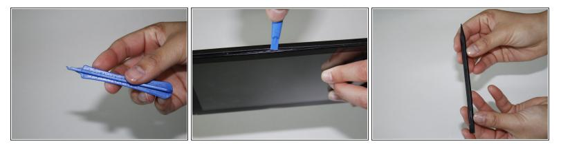
• Beginning in the upper corner of the tablet, use the blue plastic opening tool and run it along the seam. Do this slowly so you don't cause damage to the device.
