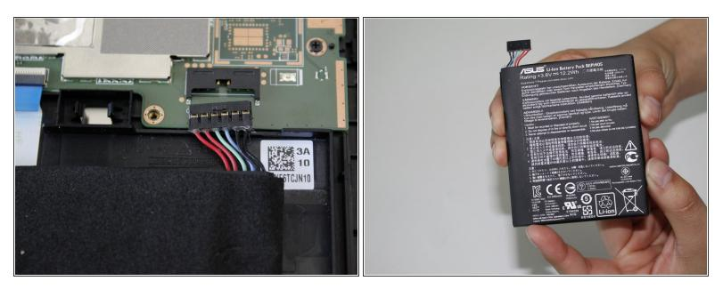
• Remove the battery from the device.
