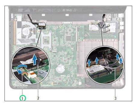
Tighten the display cable grounding screw.
