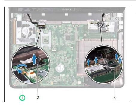
Loosen the display cable grounding screw.
