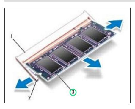
Remove the memory module(s) from the memory-module connector.
