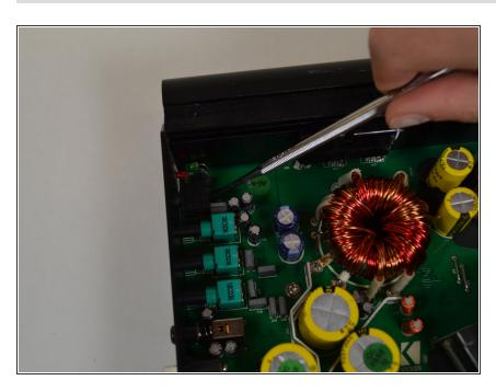
Desolder the remote receiver from the motherboard. To reassemble your device, follow these instructions in reverse order.
