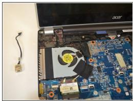
Lift the charging port up and out of the laptop.
