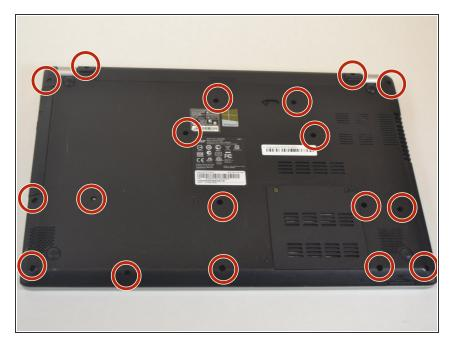
Remove the sixteen 6mm Phillips #0 screws from the bottom cover.
