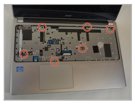
Remove the six 6mm Phillips #0 screws from underneath the keyboard.
