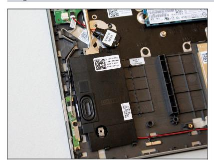
Use a metal spudger to pry off left speaker assembly.
