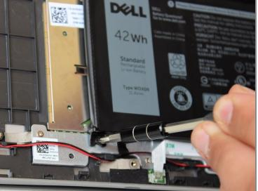
Remove the two 7.8 mm long screws on the left side of the battery with the Phillips #1 screwdriver.
