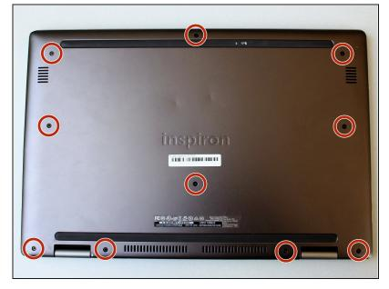
Remove the ten 7.9 mm screws with the Phillips PH0 screwdriver.
