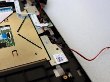
• Un-thread the wire by removing them from under the plastic clamps. No tools are required for this step. Repeat for both sides.
