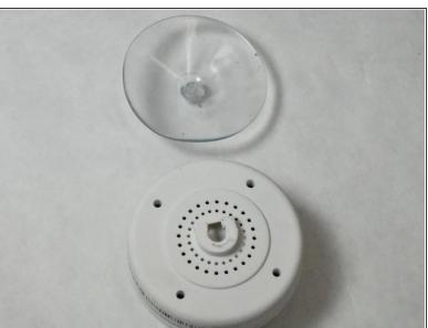
Remove the suction pad by pulling the suction out of the slot that it is in.
