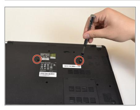
Remove the two 7mm Phillips #00 screws from the bottom of the laptop.
