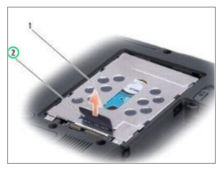
Place the hard drive assembly in the hard drive bay by aligning the tabs on the hard drive assembly with the slots in the bay and pressing the connector end down.
