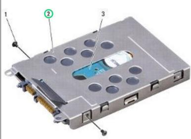
Slide out the hard drive from the hard drive assembly.
