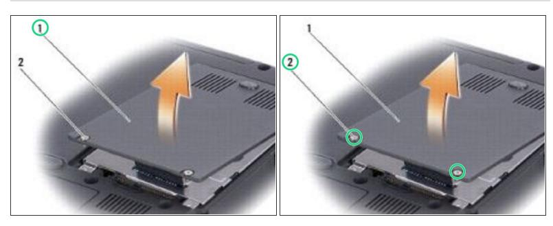
Replace the hard drive door and tighten the screws.
