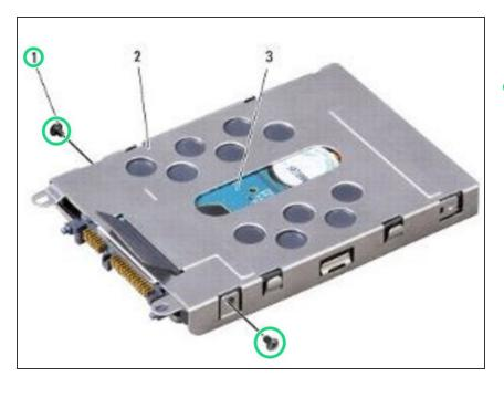
Tighten the two screws to secure the hard drive to the hard drive assembly.
