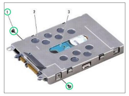
Remove the two screws securing the hard drive to the hard drive assembly.
