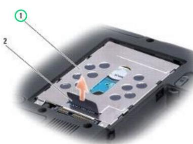
Remove the hard drive assembly using the pull-tab.
