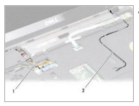
Make note of the cable routing and carefully dislodge the WLAN antenna cables and the rest of the cables from their routing guides. Pull the cables away, so that they are clear of the palm rest.
