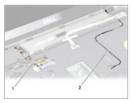
Carefully route the WLAN antenna cables into their routing guides on the palm rest and through the computer base.
