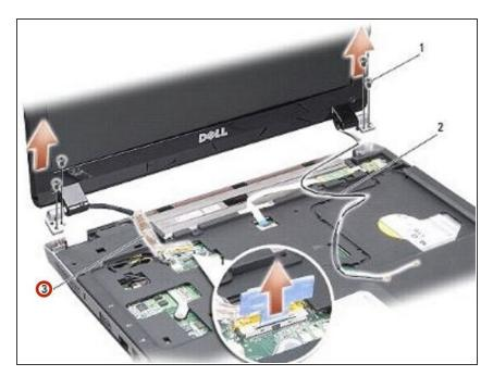
Re-route and connect the display cable to the connector on the system board.
