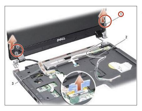
Place the **NEW** display assembly in place and replace the two screws on each side of the display hinges.
