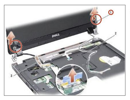
Remove the two screws from either side of the display hinges.
