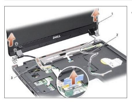
Lift and remove the display assembly.
