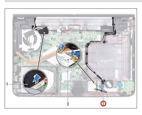
Disconnect the Mini-Card antenna cables from the connectors on the Mini-Card.
