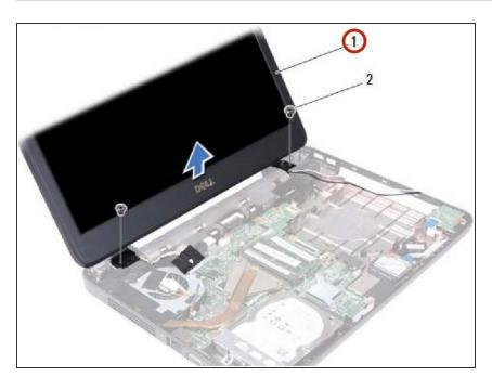
Place the **NEW** display assembly in position and replace the two screws that secure the display assembly to the computer base.
