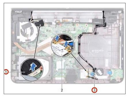
Make a note of the display cable and Mini-Card antenna cables routing and remove the cables from the routing guides.
