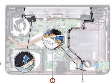
Connect the Mini-Card antenna cables to the Mini-Card.
