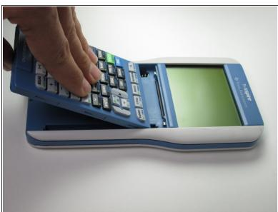
Put your hand on the keypad, slide the keypad down about a half inch, and pull up to remove the keypad.
