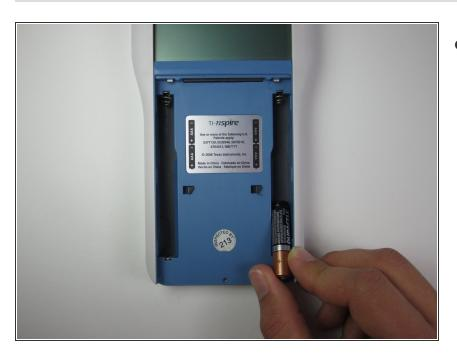
When reassembling your device, use four new batteries.
