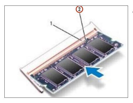
Align the notch in the memory module with the tab in the memorymodule connector.
