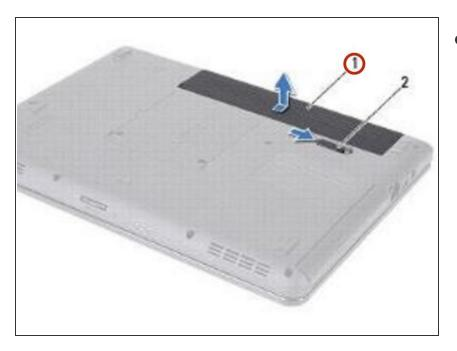
Slide and lift the battery out of the battery bay.
