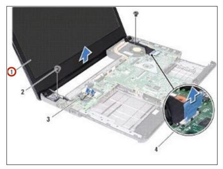
Place the **NEW** display assembly in position and replace the two screws (one on each side) that secure the display assembly to the computer base.
