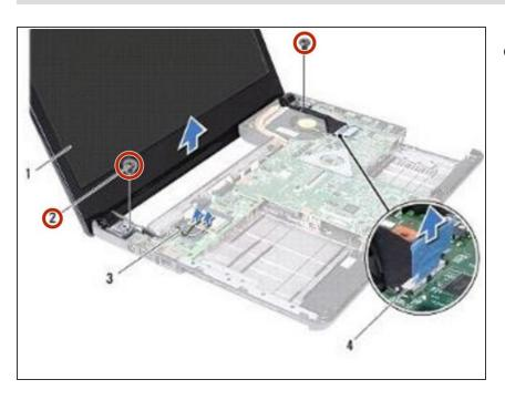
Remove the two screws (one on each side) that secure the display assembly to the computer base.
