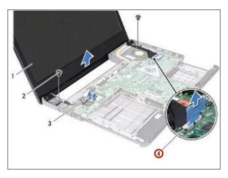
Connect the display cable to the connector on the system board.
