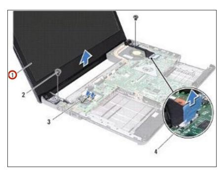
Lift and remove the display assembly out of the computer base.
