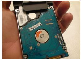
Once you've made sure all four screws are removed slide the hard drive out with your hand.
