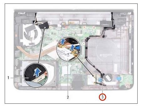
Disconnect the Mini-Card antenna cables from the connectors on the Mini-Card.
