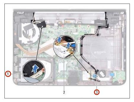
Route the display cable and Mini-Card antenna cables through the routing guides.
