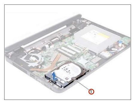
Push the hard-drive assembly towards the right to connect it to the connector on the system board.
