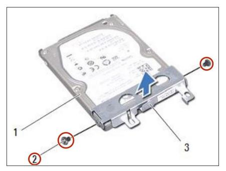
Remove the two screws that secure the hard-drive bracket to the hard drive.
