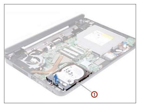
• Lift the hard-drive assembly out of the computer base.
