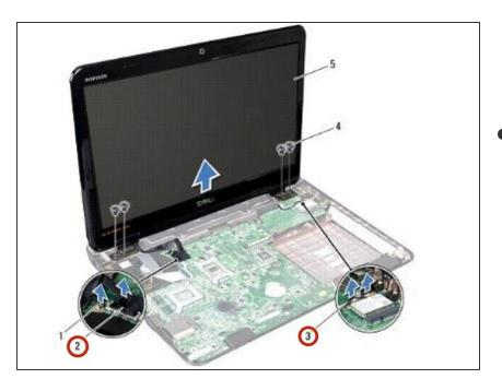
Make a note of the Mini-Card antenna cables and display cable routing and remove the cables from the routing guides.
