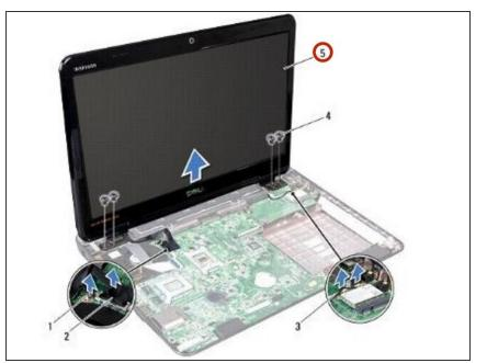
Place the NEW display assembly in position and replace the four screws (two on each side) that secure the display assembly to the computer base.
