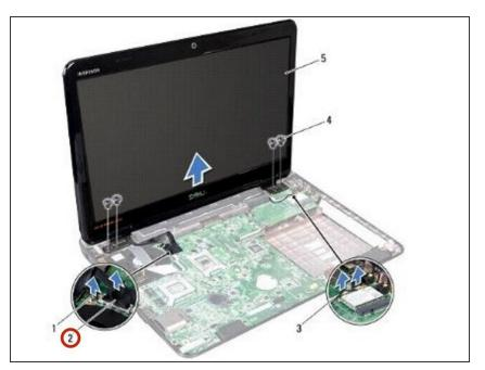
Connect the display cable to the connector on the system board, and replace the display cable grounding screw.
