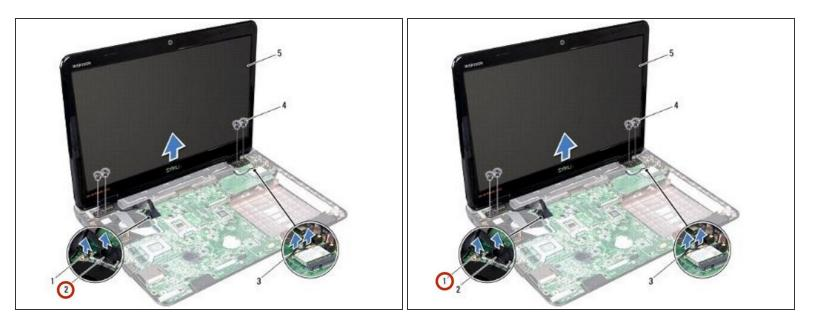
• Disconnect the display cable from the connector on the system board, and remove the display cable grounding screw.
