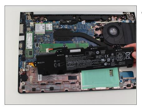
Slide the battery out and remove it from the device. To reassemble your device, follow these instructions in reverse order.
