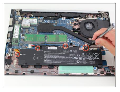
Remove the 4mm screws that are fastened on the battery with your T9 Torx screwdriver.
